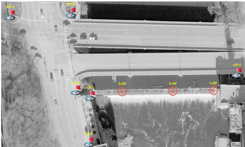
Image from survey marker layout on similar dam project
